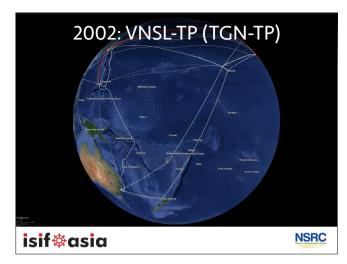
2002 brings the decommissioning of ANZCAN and the introduction of VNSL Transpacific (A project begun as Tyco Transpacific, and now now known as TGN TransPacific), nominally a US Japan cable. It was planned and implemented as a 5 terabits per second cable, another step change for capacity in the Pacific.
