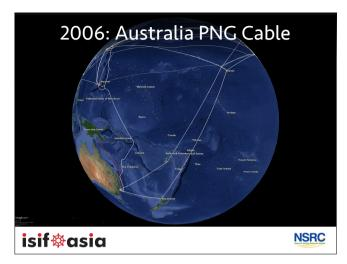
2006 has the cold, dead snake of PacRim West dragged off the seafloor and hauled to Port Moresby - recommissioned with a design bandwidth of just over a gigabit per second. From what I understand, regeneration in this cable is electronic, not optical, and E5 (565mbps) is as fast as electronic regeneration will work. So we've got two 565mbps pairs bringing a total of 1.1 gigabit per second into PNG.
