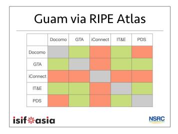
Here's the results of a set of traceroutes between the various carriers in Guam. We can see that not all of Guam's carriers interconnect locally - and some, like iConnect, send all of their traffic directly to the United States, not peering any of it on-island.
