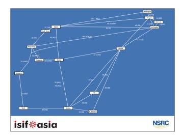
I've constructed a simple model of cables in the Pacific and network latencies to look at how Guam connects to the rest of the world. Providing the best performance for real-time tasks like Skype, Facetime, and distance learning applications means keeping latency down.
