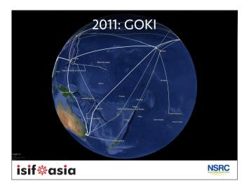
In 2011 we remove at least some of TPC-5 from service, and add a half-new cable called GOKI. 80gbps reported. What needs a direct path from Guam to Okinawa to Korea? I can think of one customer looking for a low latency path controlled by AT&T the whole way. Are any commercial providers using it? No idea.
