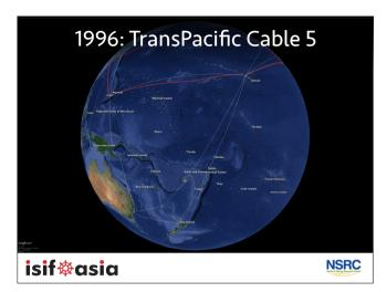
In 1996 TPC 5 lights up two pairs at 5gbps each (2x STM-16, with 32 155mbps circuits available) in a loop connecting the US, Hawaii, Guam, and Japan. That's starting to sound like real capacity, at least for the 90s. Note Hawaii and Guam both starting to become important waypoints.
