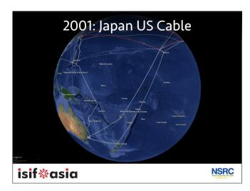
And a top-up for Hawaii in 2001, as a new cable from the US to Japan passes through with 320 gigabits per second. Hawaii - or at least O'ahu, is now as busy as Guam when it comes to cables. Capacity was doubled in 2008.
