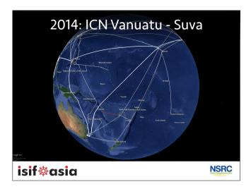
and last one, the ICN cable from Vanuatu to Fiji in 2014. While both were deployed with initial capability of 20gbps, neither has more than a few hundred mbps in use.
