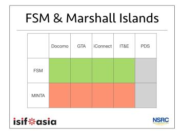
Here's the results of a set of traceroutes from Guam carriers to the Federated States of Micronesia and to the Marshall Islands. PDS is not represented here as they do not host a RIPE Atlas Probe, and MINTA's RIPE Atlas probe has been offline for many months.
